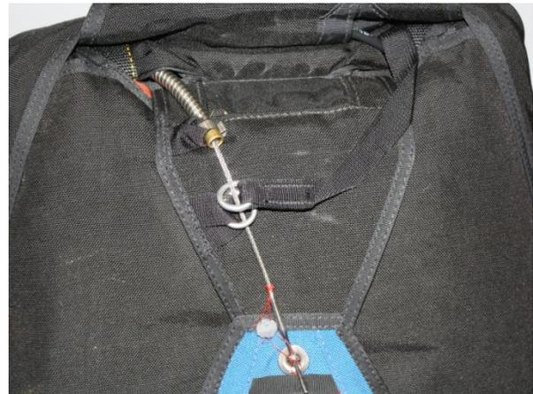
**Reserve Closing Loop** – Check that the loop does not have any fraying and that the reserve pin is the only item passing through it.
