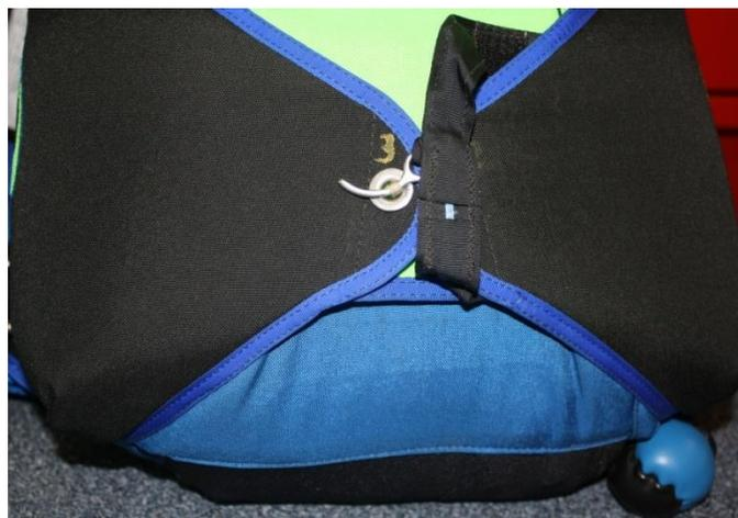
**Pilot Chute** – You should not be able to see much if any pilot chute material when it is packed into the BOC pouch. The main deployment handle should be out of the pouch and easily accessible.
