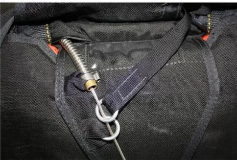
To disconnect the RSL, pull on the red tab to release the silver fitting from the silver ring on the back of the right riser group. To re-connect the RSL, place one end of the hook through the ring, pull on the red tab with one hand while you squeeze the two parts of the hook together and then release the red tab. Make sure the hook is locked in place. Feel free to try this on your own.
