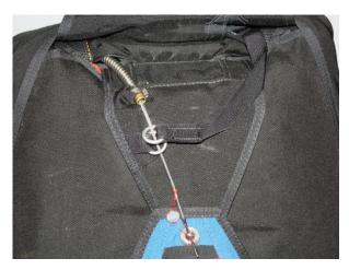
**Reserve Pin** – Check to ensure that the pin is 3/4 of the way through the closing loop.
