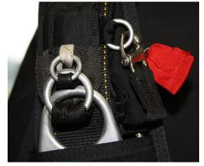
**Reserve Static Line (RSL)** – The RSL should be hooked up to the small silver ring on the right riser
