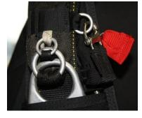
the 3-ring system. It is then routed over the right shoulder without being routed around anything, over the Cypres control unit cable, under the reserve flap, and has the reserve cable passing through the silver ring at the end of it. The RSL does **not** disconnect the main parachute.
