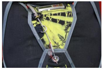
**Rigger's Seal** – Check to make sure that the red thread is fastened above the flatter end of the reserve pin and below the closing loop. The red thread should have some slack so that it does not break too easily, but not so much that you can slip it off the end of the pin. The thread should pass through the gray seal of the rigger. The seal must have an identifiable mark on it that lets you know which rigger packed the reserve.
